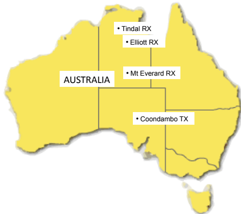
Fig. 4. Geographic layout for MSE-I shown on the map of Australia. The experiment used equipment located at Coondambo (Tx array, OIS Tx and clear channel advice receiver), and receiver systems located at Mt Everard (863km), Elliott (1514km) and Tindal (1864km). The total ground-range depth between the nearest and furthest receiver system is approximately 1000km and all receiver locations have similar orientation with respect to the transmitter array. Precise range, bearing and azimuth details for both campaigns are given in table I.
