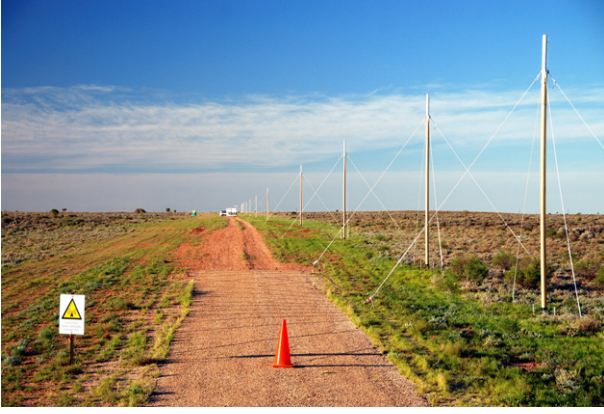
Fig. 7. End aspect photograph showing the 12 element minimum redundancy array used in the Mode Selection Experiment. The total aperture length was 1200m and the array was oriented with end-fire at a bearing of 359.5^\circ T. The photo is taken from the southern end of the array looking north. The white equipment shelter just visible on the horizon contained the transmitter equipment and the central control system for the experiment. It was located mid-way along the array.
