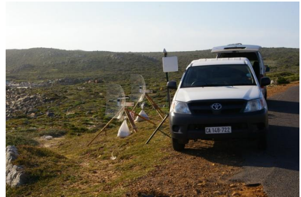
Fig. 3. NetRAD transmit/receive node, showing separate radar transmit and receive antennas, and GPS and wireless link antennas.
