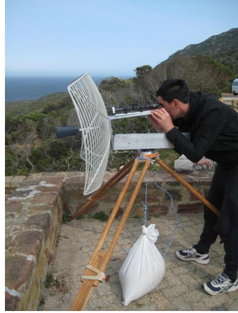
Fig. 2. Close-up of NetRAD radar antenna. The azimuth/elevation mount allows a pointing precision of better than \pm 1^\circ . The beamwidth in both planes is approximately 10^\circ .
