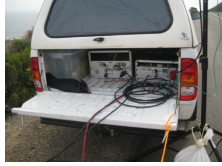
Fig. 1. NetRAD hardware for one node deployed in a truck.
